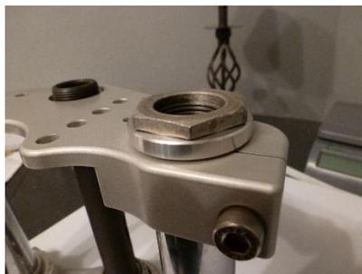
**Install the stanchion top bolt/nut and TT spacer. The spacer should be sitting on top of the fork tube to seal it.**
