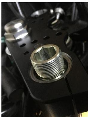
Install the center stem nut and tighten to about **40 ft/lbs to seat it**. The recess should remain the same in both clamp bores. Photo shows top stack for 86-on model.
