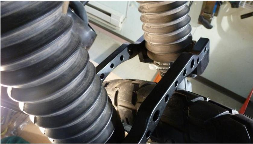
Install the 8, 6mm screws from the bottom into the bridge pegs.
