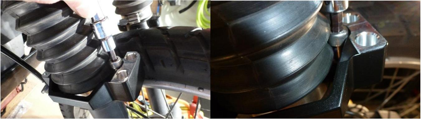
Note the two bridge pieces have a side with radiused edge and a flat side. **The flat side goes IN** so the ToasterTan logo can be read facing out. Drop the bridge pegs into the holes and wiggle down so it seats flat. It's OK if they are snug and don't go all the way down. You can pull them in with the fastener – just be sure they are in far enough so they don't wedge sideways in the bore.
