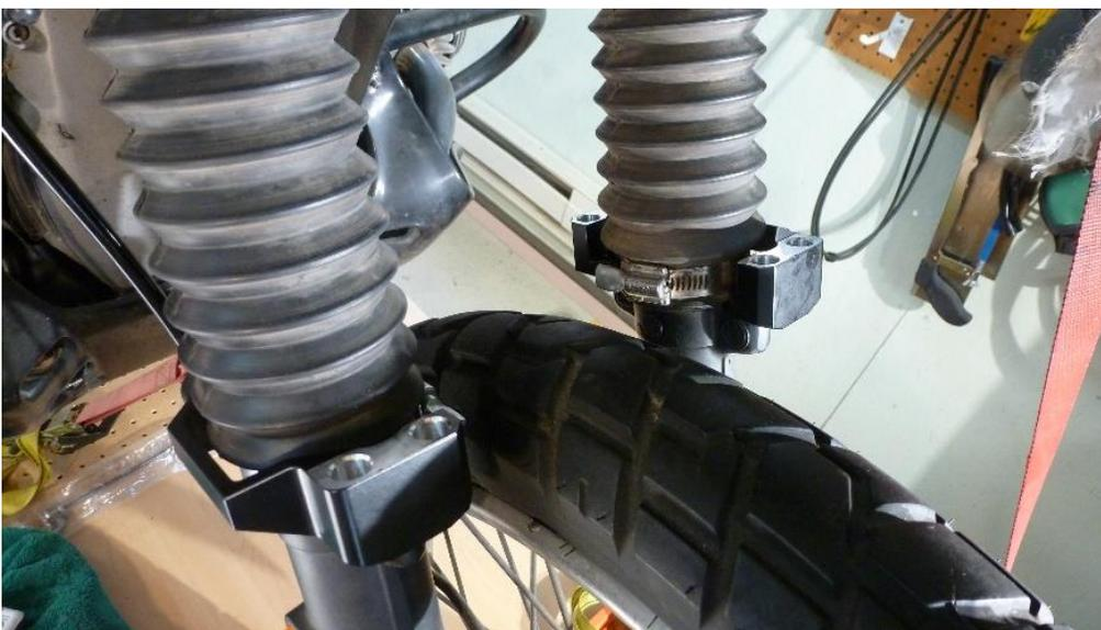
Pull the boot back against the fork tube and be careful not to pinch the boot rib under the bolt washer. I found using a socket/allen works best as the allen wrench L would hit the boot when turning in.
