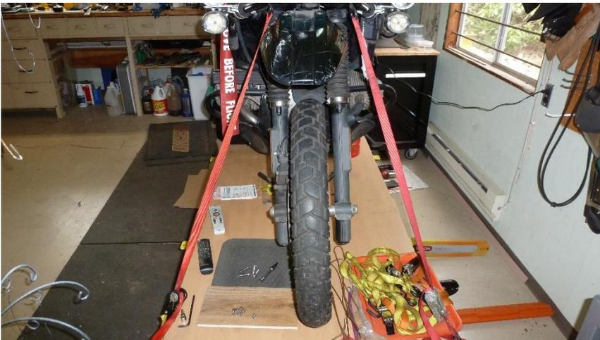
Look at the bridge from the front and align it to be centered in the slotted mounting holes. Cross-tighten the bolts on each side: one on the front left – then the right rear / right front – left rear. Make them snug enough the bridge doesn't move. Then torque to 18 ft/lbs. You don't really need blue Loctite, but it won't hurt. Again: small amount. Take it for a test ride to feel for stiction.
