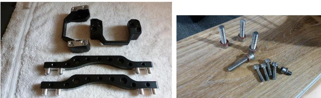
First – rotate any boot clamps so the tightening adjuster is on the inside of the forks. This is so you can access them with the bridge in place. Set the two bases on the fork boss with shiny side up and loosely screw in the bolts. Leave them loose enough so you can wiggle the bridge piece on and move the base around to adjust.
